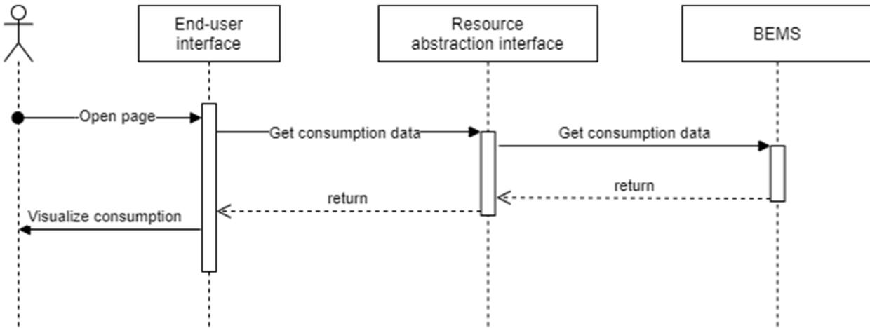
Figure 10: Sequence diagram of energy consumption monitoring use case.
