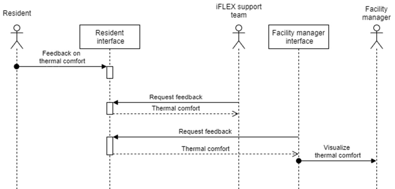
Figure 8: Sequence diagram for feedback on thermal comfort.
