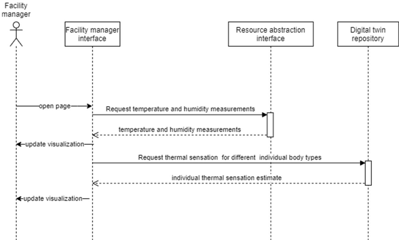
Figure 7: Sequence diagram for collecting and visualizing thermal comfort related data.
