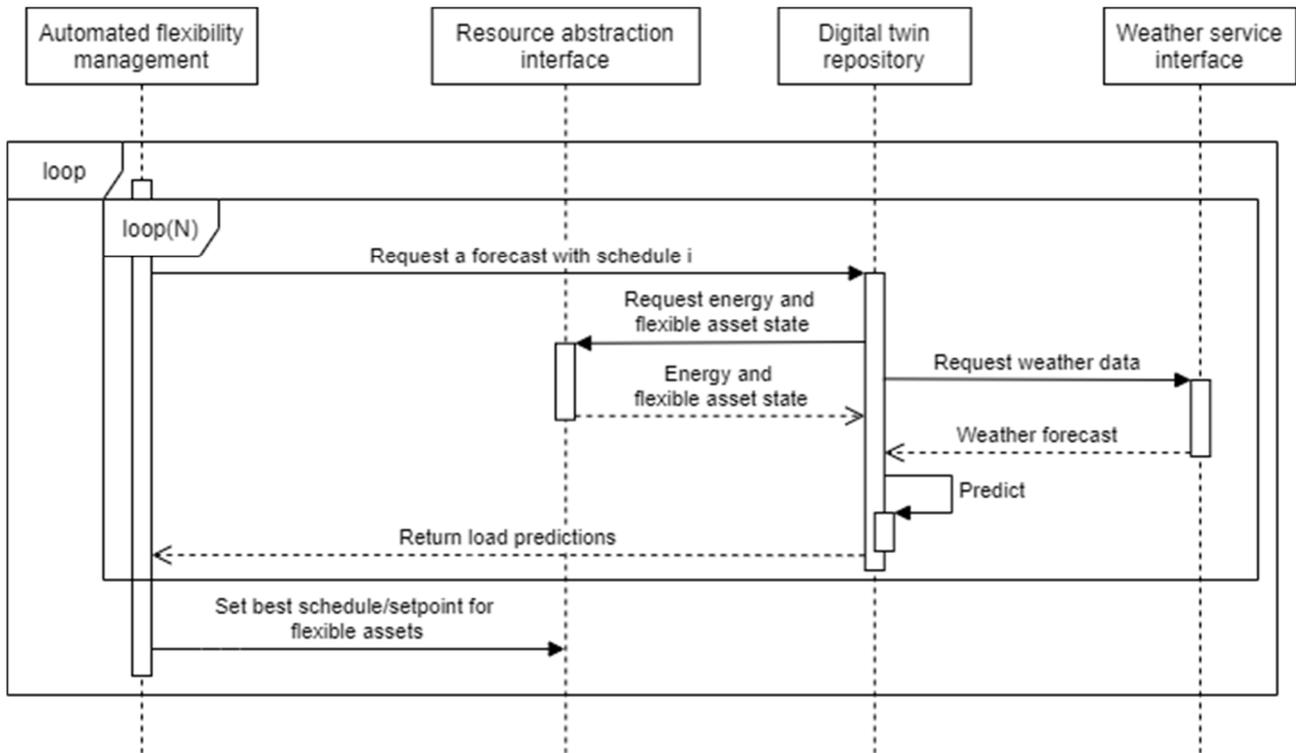
Figure 13: Sequence diagram of schedule optimization for flexible assets.
