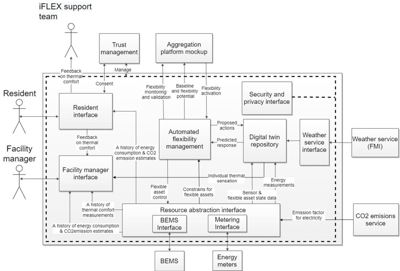
Figure 6: Functional view of the iFLEX Assistant to be customized for the apartment building (FIN pilot).
