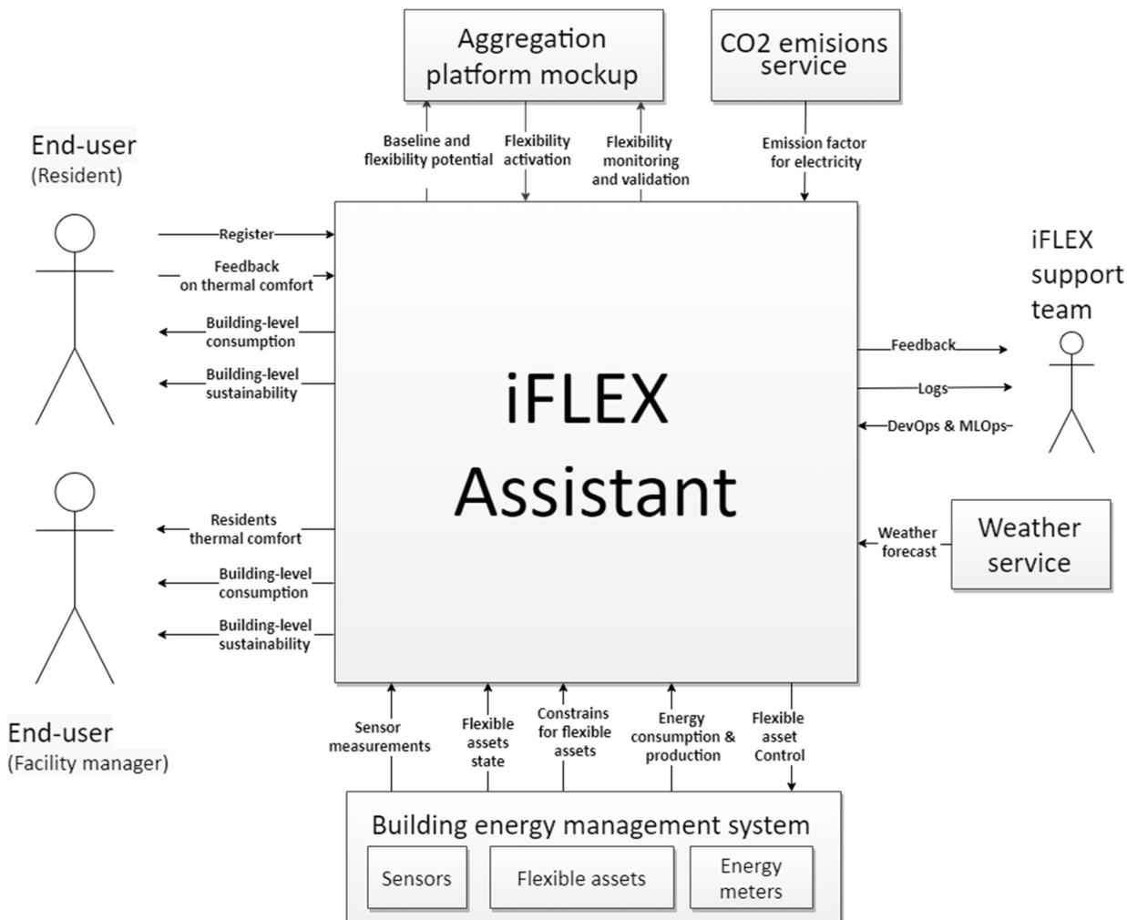
Figure 5: Context view of the iFLEX Assistant to be customized for the apartment building (FIN pilot).
