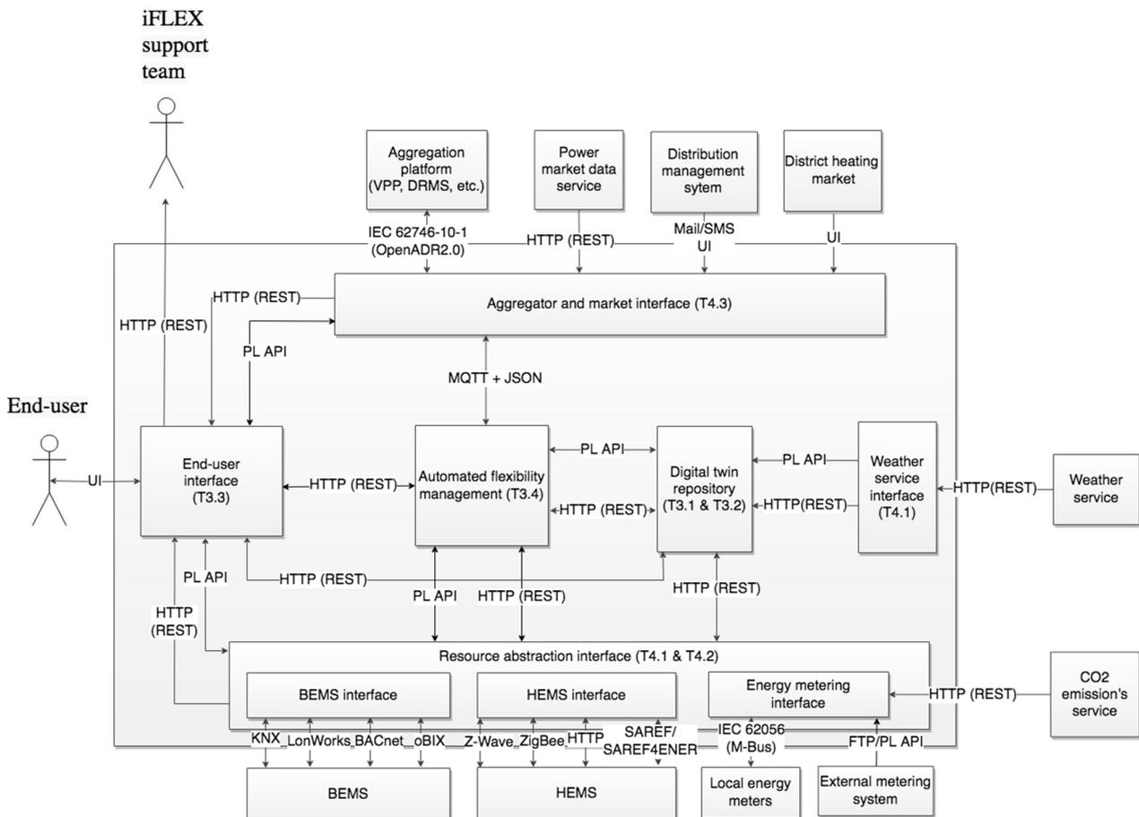
Figure 4: Mapping of the interoperability technologies to the functional architecture of the iFLEX Framework.
