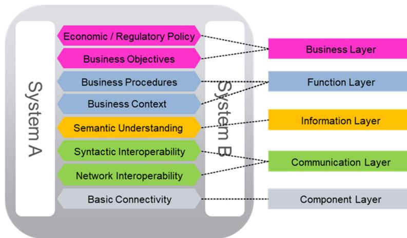
Figure 3: Interoperability dimensions of SGAM [7].
