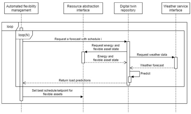
Figure 13: Sequence diagram of schedule optimization for flexible assets.
