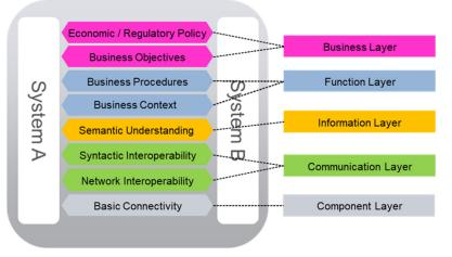
Figure 3: Interoperability dimensions of SGAM [7].
