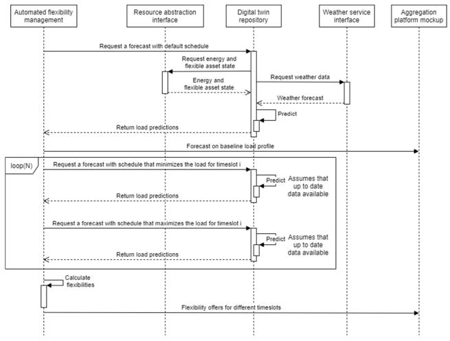
Figure 11: Sequence diagram for the offer flexibility use case.
