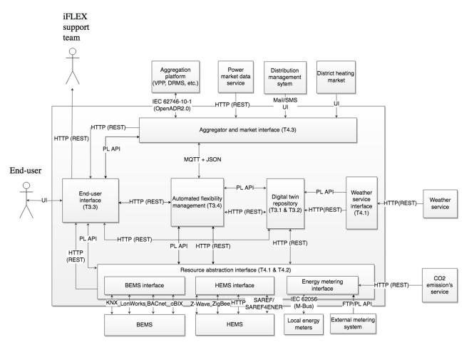
Figure 4: Mapping of the interoperability technologies to the functional architecture of the iFLEX Framework.
