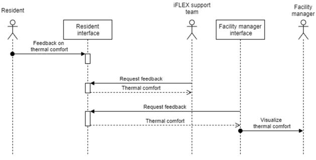
Figure 8: Sequence diagram for feedback on thermal comfort.
