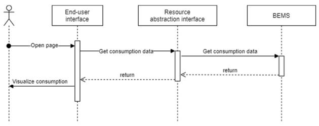
Figure 10: Sequence diagram of energy consumption monitoring use case.
