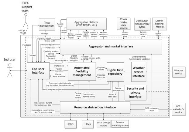
Figure 2: Functional view of the common iFLEX Framework.
