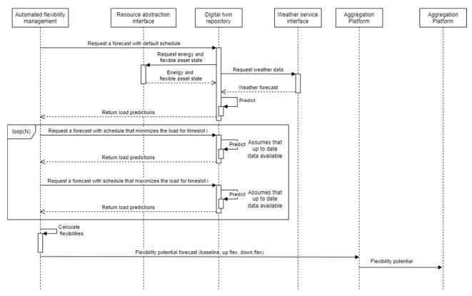
Figure 39: Sequence diagram for the offer flexibility use case.
