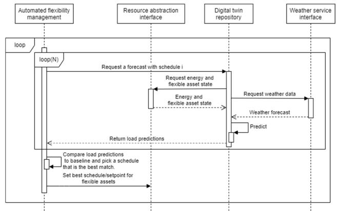
Figure 42: Sequence diagram of schedule optimization for flexible assets.
