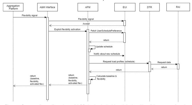
Figure 30: Sequence diagram illustrating explicit DR signal and schedule optimization with explicit acceptance from the End-user.
