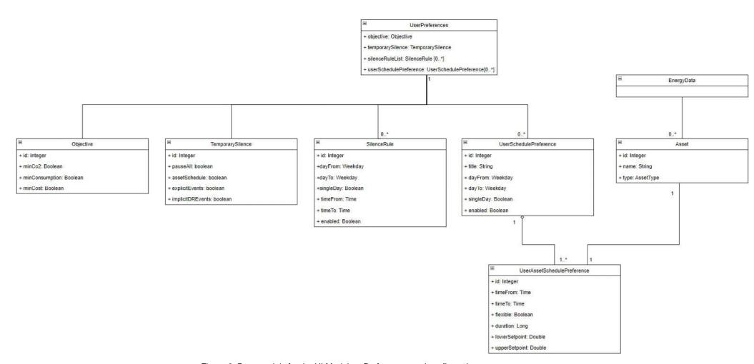
Figure 8: Data models for the UI Module – Preferences and configurations.
