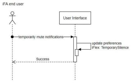
Figure 20: PUC-1 sequence diagram, scenario: Temporarily mute notifications.
