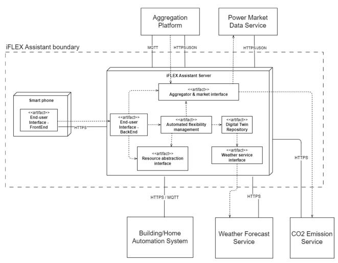
Figure 13: Example deployment view of an iFLEX Assistant based on the iFLEX Framework.
