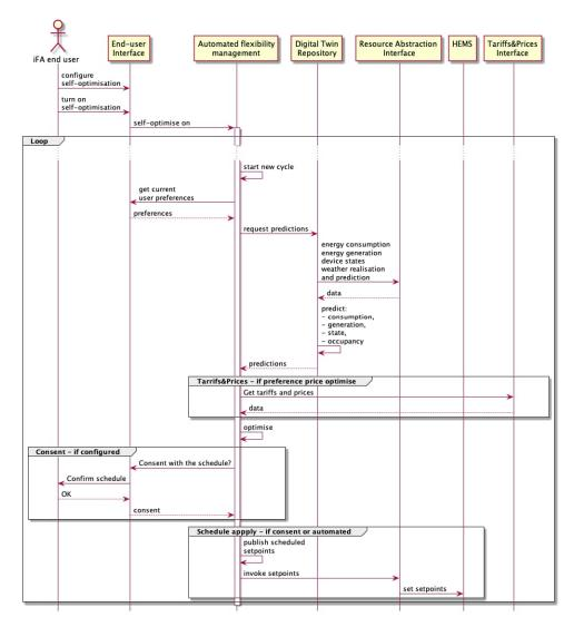
Figure 32: Increase self-balancing through forecasting and automation.
