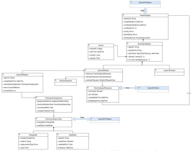
Figure 3: Data models for the A&M Interface Module – Flexibility Signal, Validation Data, and Report.
