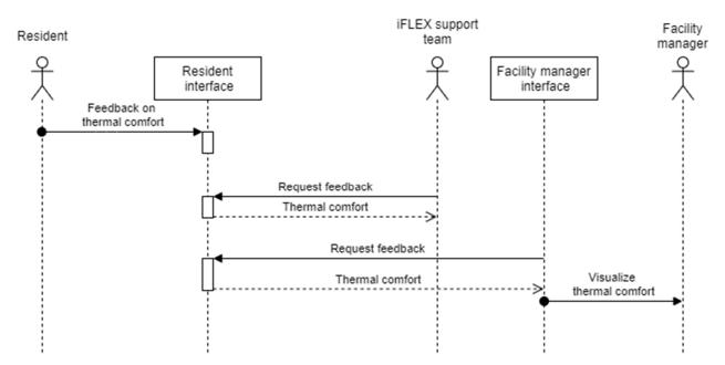
Figure 36: Sequence diagram for feedback on thermal comfort.
