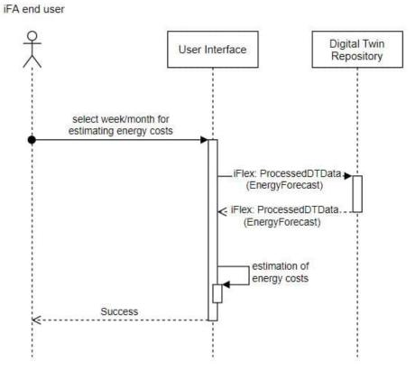
Figure 23: PUC-4 sequence diagram, scenario: Estimate energy costs.
