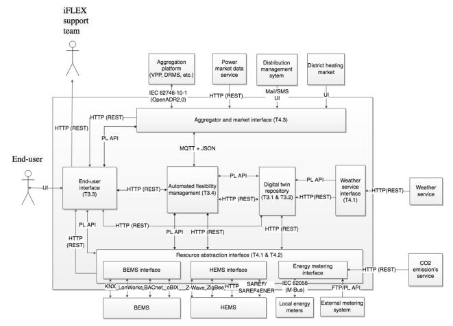
Figure 15: Mapping of the interoperability technologies to the functional architecture of the iFLEX Framework.
