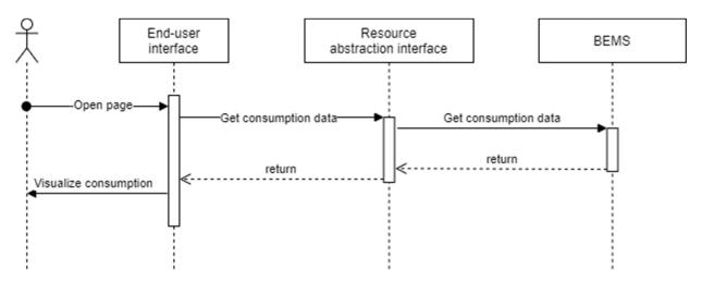
Figure 38: Sequence diagram of energy consumption monitoring use case.
