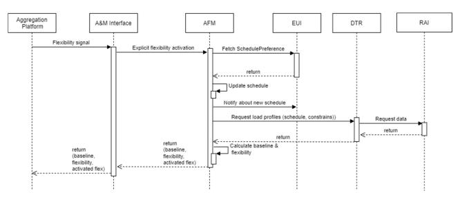
Figure 29: Sequence diagram illustrating explicit DR signal and schedule optimization without a need for explicit acceptance from the End-user.
