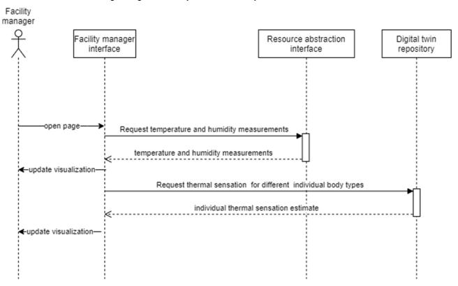
Figure 35: Sequence diagram for collecting and visualizing thermal comfort related data.
