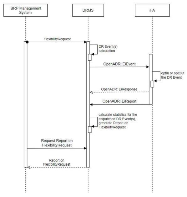
Figure 44: Sequence diagram for activating flexibility and generating report on flexibility request in the Greek pilot.
