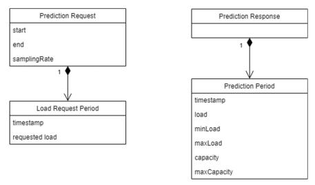
Figure 6: Data models for Digital Twin Repository interface.
