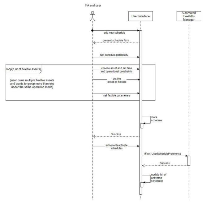
Figure 18: PUC-1 sequence diagram, scenario: Set flexible schedules of assets.
