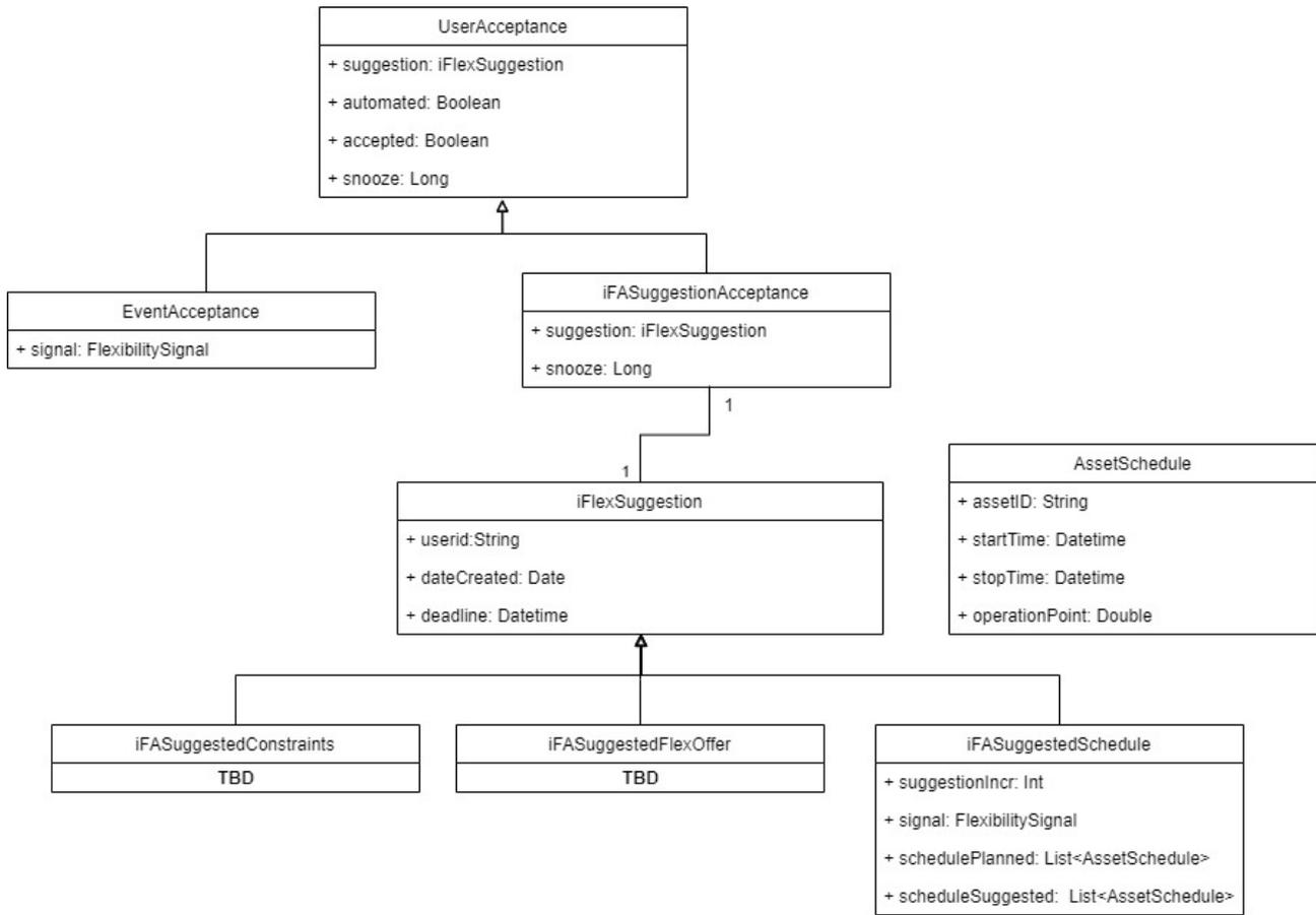
Figure 26: Class diagram of iFLEX Suggestions
