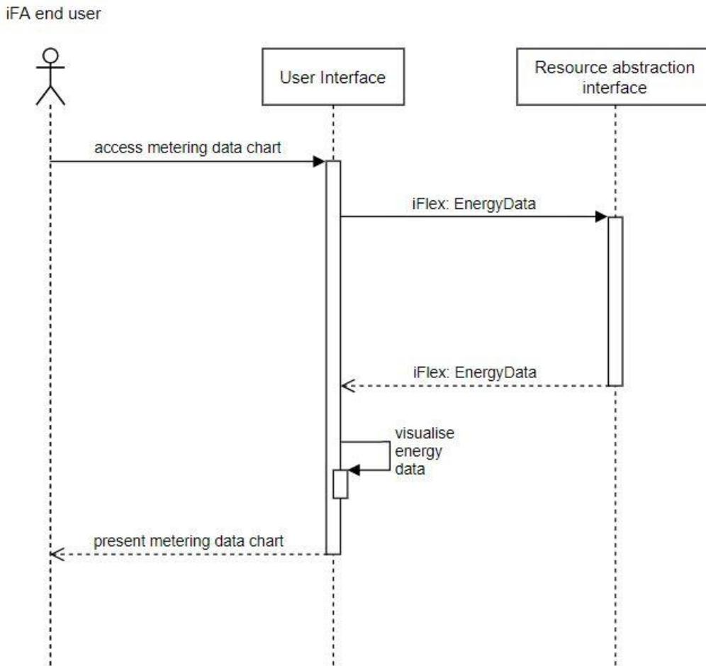
Figure 19: Sequence diagram of SUC-9 - Access real-time energy data
