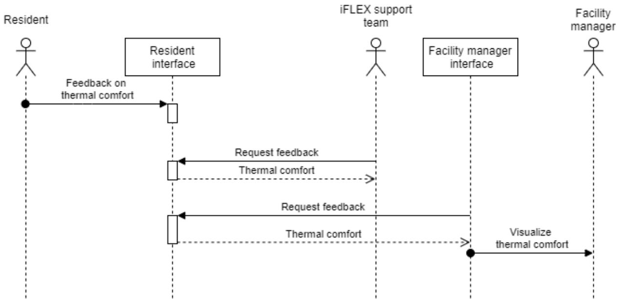
Figure 24: Sequence diagram of SUC-14 - Provide feedback on thermal comfort
