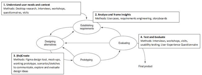
Figure 1: iFLEX design process model using 'A simple interaction design lifecycle model' by [2], p. 332, fig. 9.3
