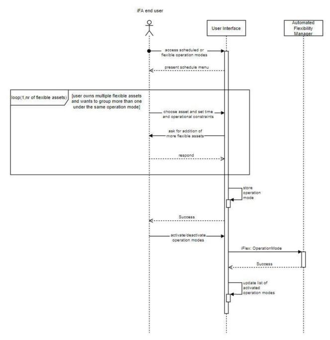
Figure 23: Sequence diagram of SUC-13 - Define comfort levels, Scenario: Set schedules of flexible assets
