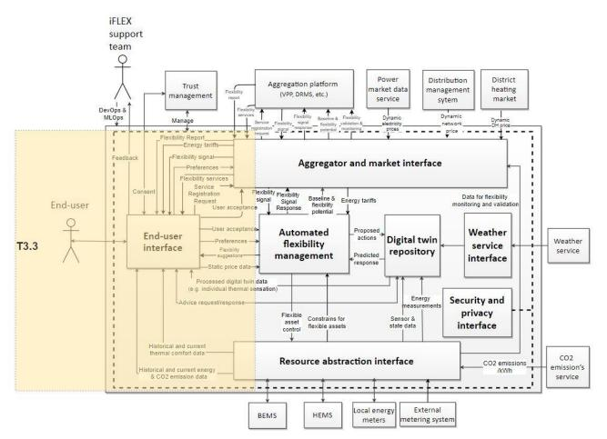
Figure 3: Functional view of the common iFLEX Framework [9]
