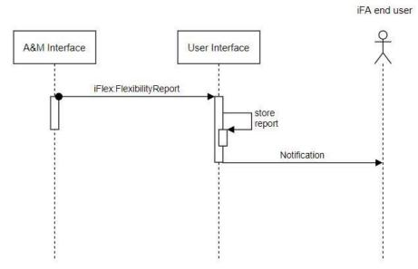
Figure 22: Sequence diagram of SUC-12 - Present reports, Scenario: Receive new flexibility report
