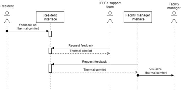
Figure 24: Sequence diagram of SUC-14 - Provide feedback on thermal comfort
