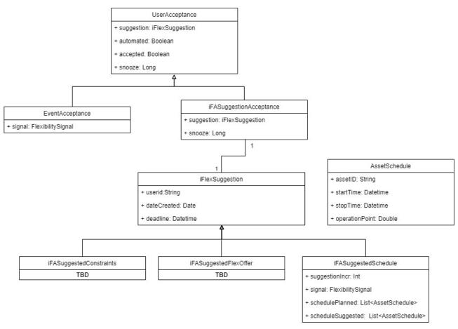
Figure 26: Class diagram of iFLEX Suggestions
