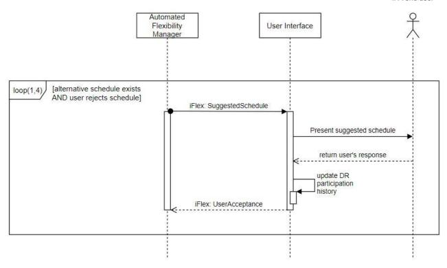
Figure 21: Sequence diagram of SUC-11 - Grant acceptance to schedules, Scenario: Manual operation
