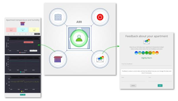
Figure 30: The User Page: Apartment Temperature and Feedback
