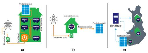
Figure 13. Three different cases suggested by the smart grid working group for Finland [18]. A) EC within a housing company, b) EC crossing property boundaries, c) distributed EC
