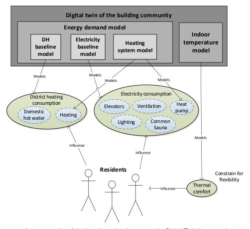
Figure 9: Conceptual representation of the interdependencies among the Digital Twin (measured parameters (green), non-measured parameters (blue)) and the residents of the building community.
