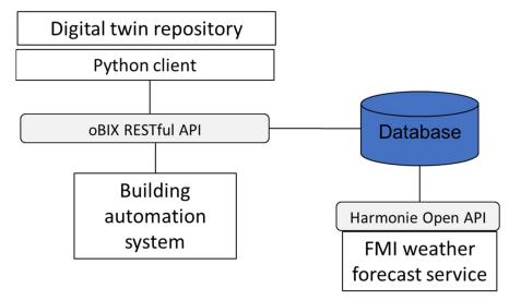
Figure 11: Weather forecast interface module integrated into the Resource abstraction interface component.
