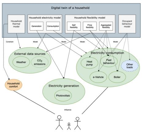
Figure 10: Household modelling (models in grey, measured parameters in green, constraints in orange, non-measured parameters in blue). Full arrows represent phase one focus.
