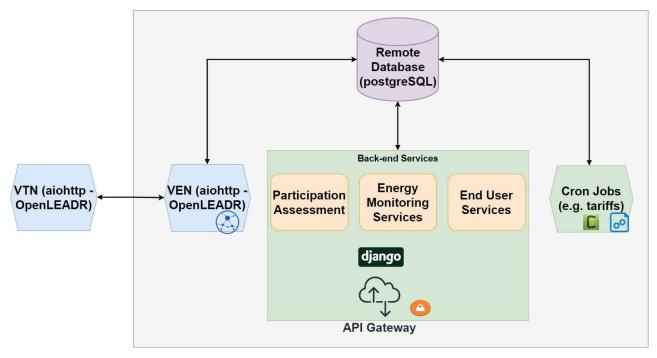
Figure 4: Technology stack of A&M's Interface module for the residential iFA
