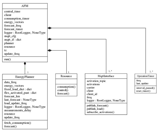
Figure 8: UML class diagram for the Automated Flexibility Manager.
