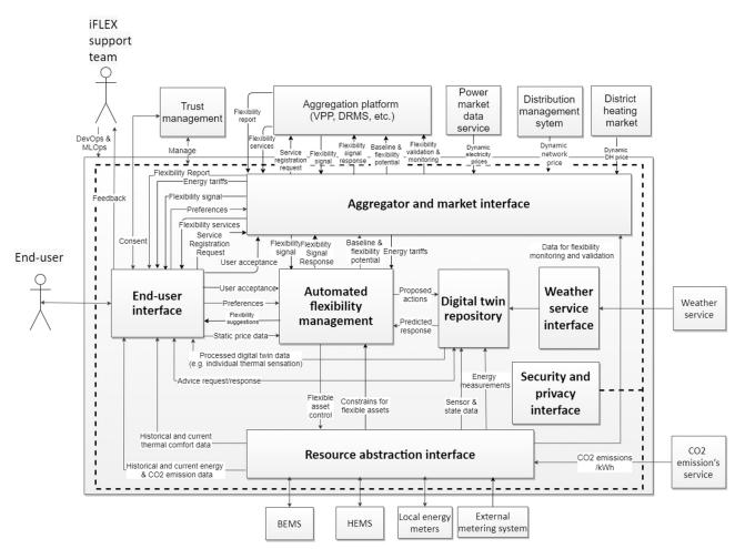
Figure 2: Functional view of the iFLEX Framework.
