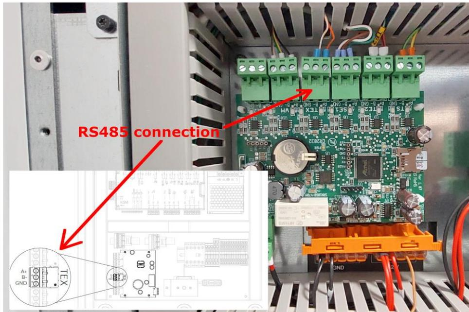
Figure 11: RS485 connection to Kronoterm KSM main unit
