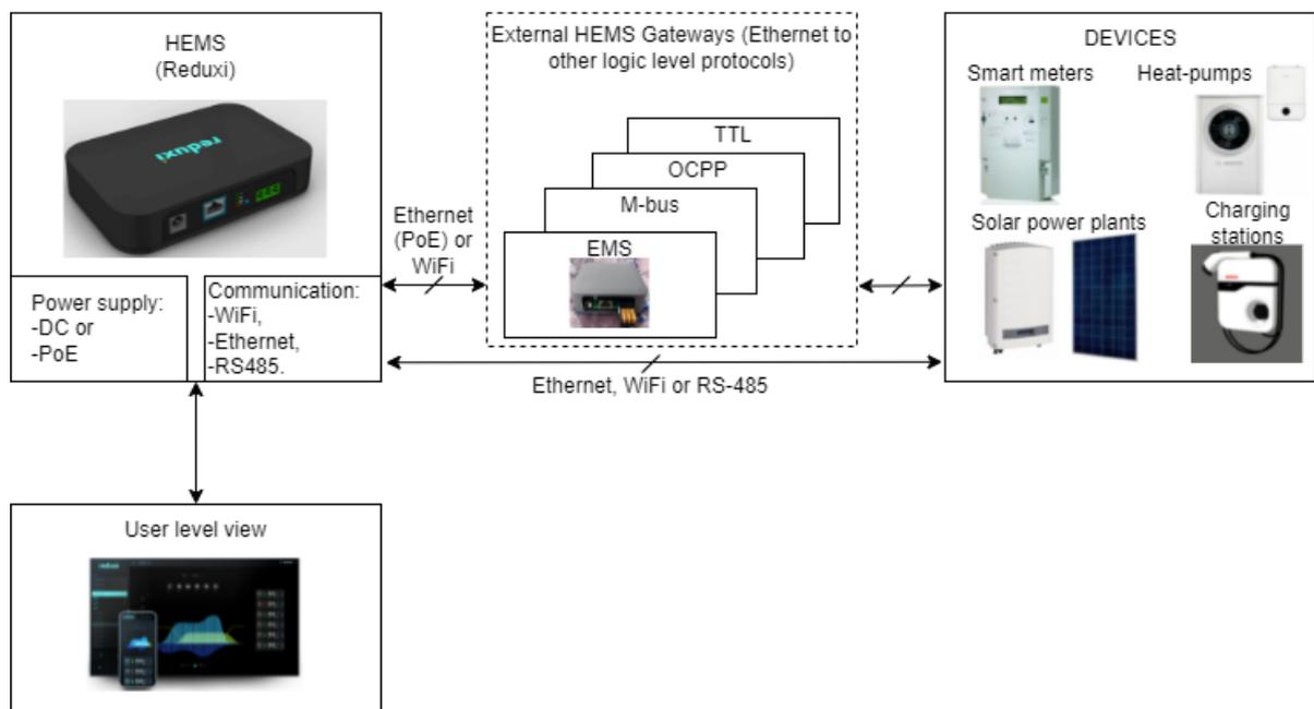
Figure 10: Connection of the HEMS with end user devices
