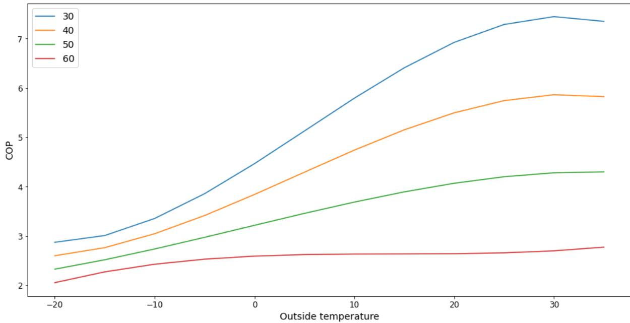
Figure 17: BOSCH Compress 6000 AW 9 heat pump COP parameters model. The curves present characteristics at different inlet water temperature
