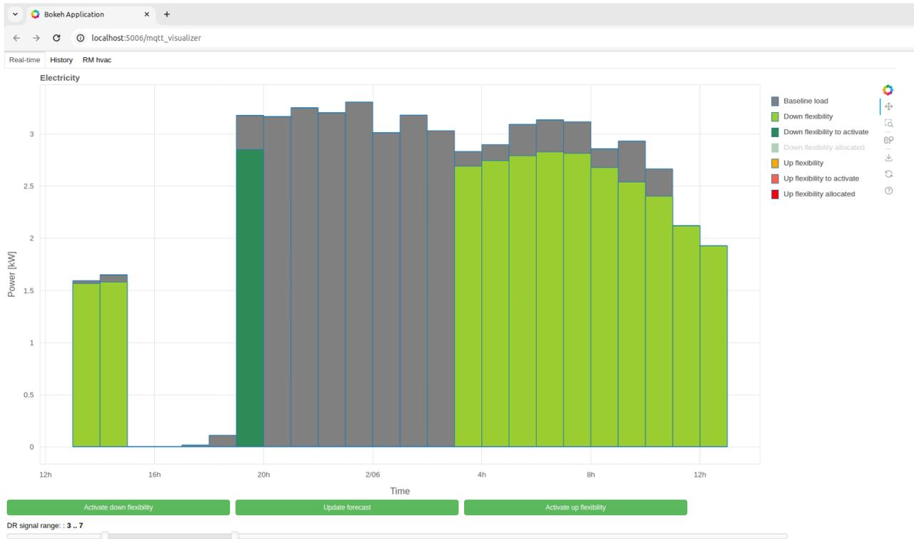
Figure 20: Visualisation of the forecasted baseline and flexibility after flexibility request has been received by the AFM
