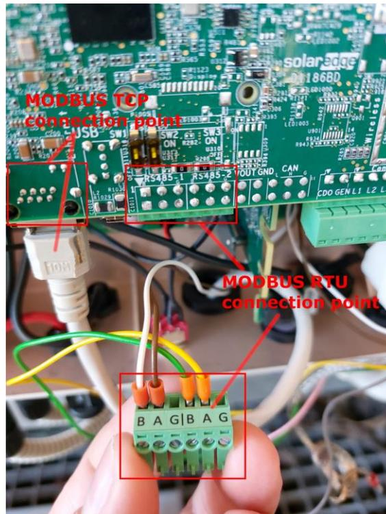
Figure 13: The connection point for the HEMS unit to the self-sufficient supply solar power plant via SolarEdge Modbus RTU communication protocol
