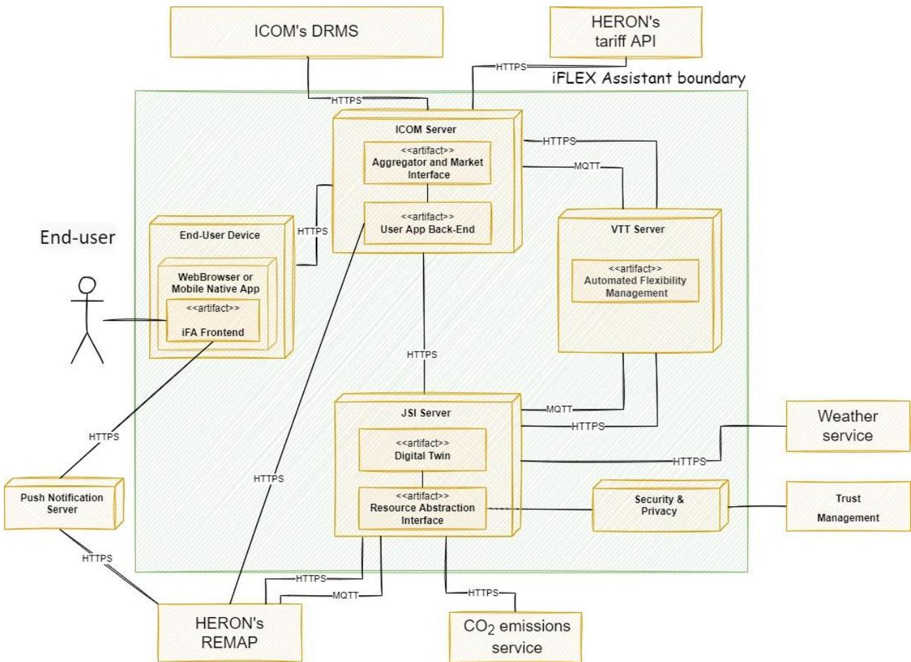
Figure 6: Deployment view of iFA for Phase 3 of the Greek pilot
