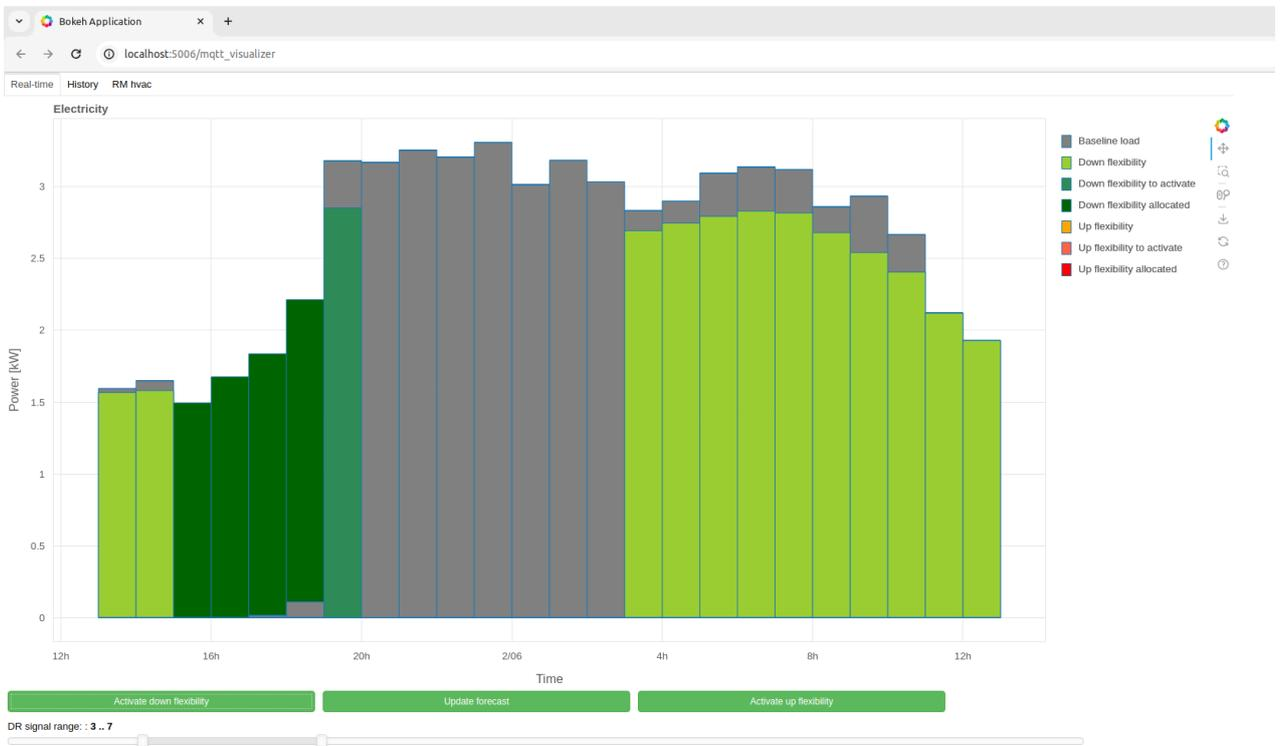
Figure 19: Visualisation of the forecasted baseline and flexibility after flexibility request has been received by the AFM
