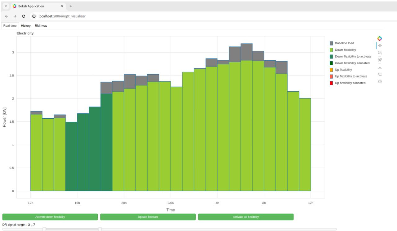
Figure 18: Visualisation of the baseline and flexibility potential provided by the AFM.
