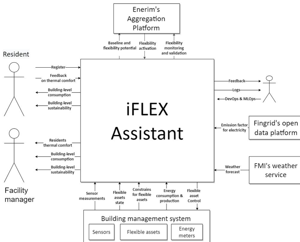
Figure 1: iFLEX Assistant of the apartment building pilot with relevant stakeholders and external systems
