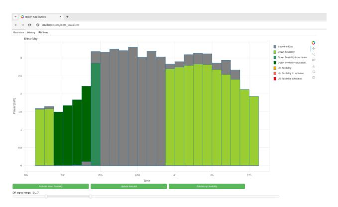
Figure 19: Visualisation of the forecasted baseline and flexibility after flexibility request has been received by the AFM Flexibility period to be activated is represented in dark green. Notice the "rebound" effect after the DR event in which the energy is paid pack according to the law of energy conversion.
