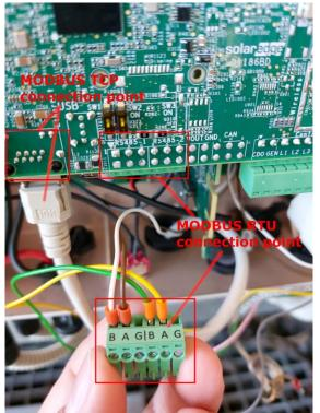
Figure 13: The connection point for the HEMS unit to the self-sufficient supply solar power plant via SolarEdge Modbus RTU communication protocol
