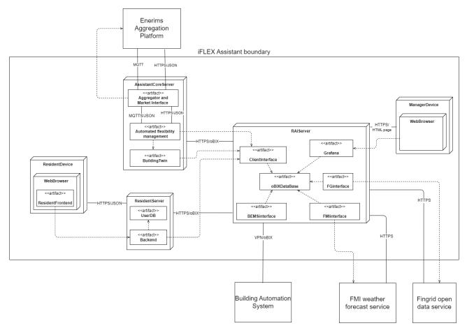
Figure 2: Deployment view of the iFLEX Assistant prototype for the apartment building iFLEX Assistant.
