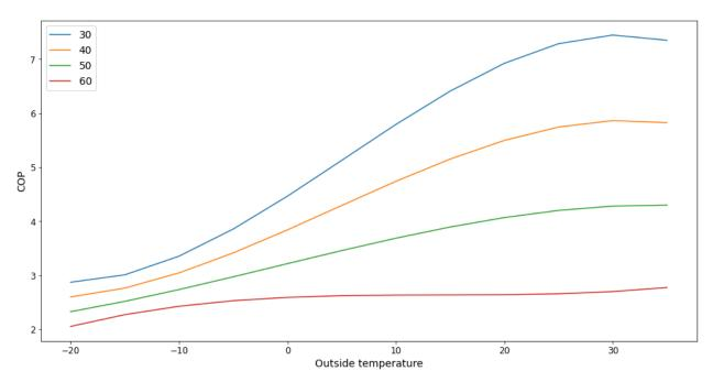
Figure 17: BOSCH Compress 6000 AW 9 heat pump COP parameters model. The curves present characteristics at different inlet water temperature
