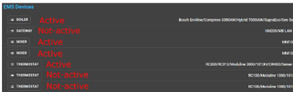
Figure 14: Active and inactive devices on the EMS bus
