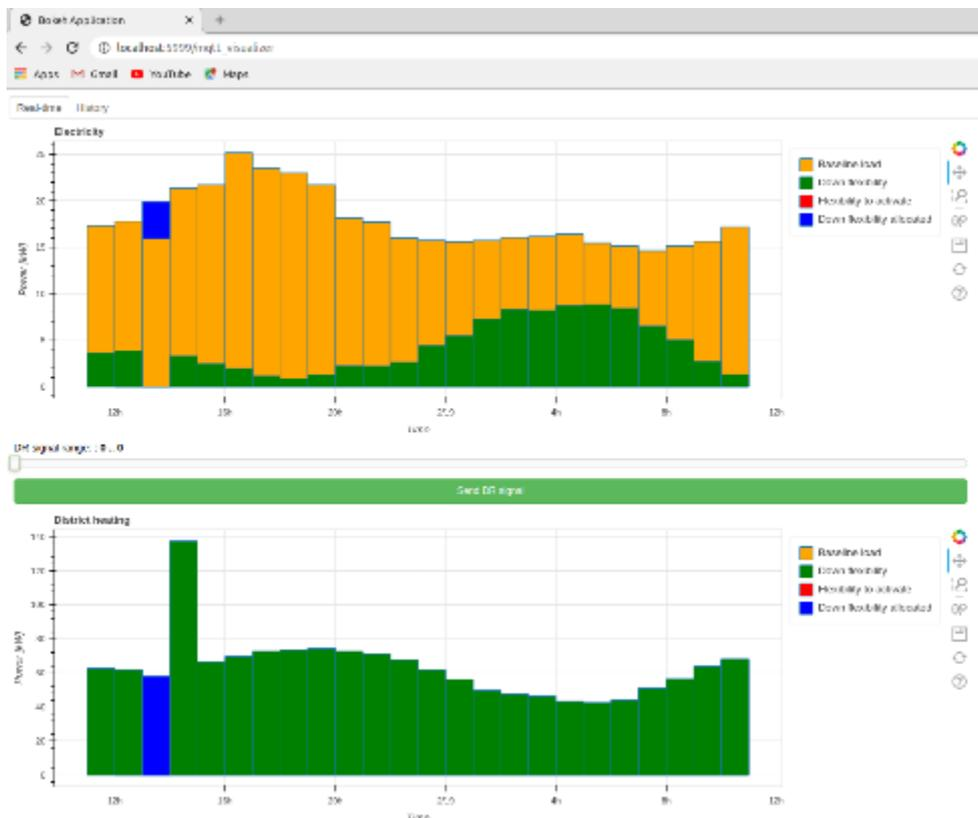
Figure 23: Demonstration interface visualizing the baseline and flexibility forecasts for electricity and district heating in the Finnish pilot building. The flexibility for period from 13:00 to 14:00 ECT was activated for both electricity and district heating vectors
