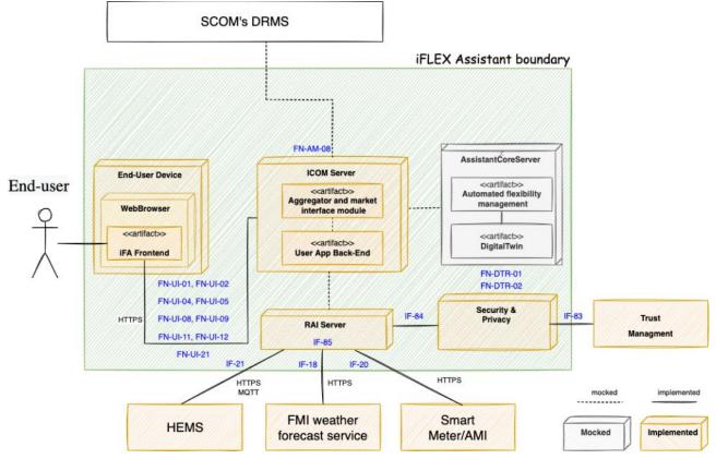
Figure 105: Technical Validation: Deployment diagram of the Slovenian pre-pilot
