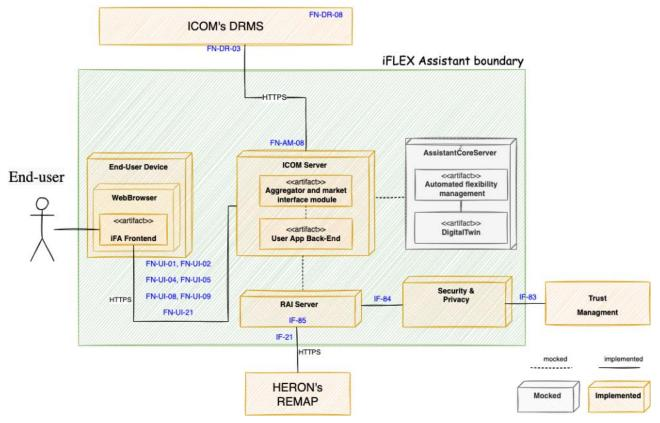
Figure 104: Technical Validation: Deployment diagram of the Greek pre-pilot
