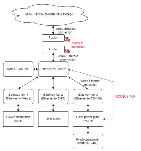
Figure 11: Flowchart of the installed devices (second manufacturer)
