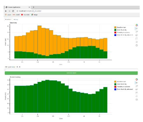
Figure 22: Demonstration interface visualizing the baseline and flexibility forecasts for electricity and district heating in the Finnish pilot building
