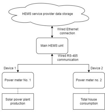
Figure 8: Flowchart of the installed devices (first manufacturer)
