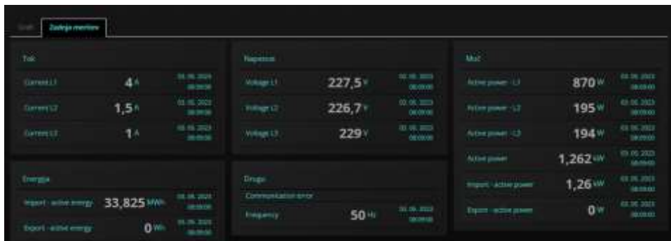
Figure 9: Numerical display of the total building consumption from the Iskraemeco AM550 distribution meter
