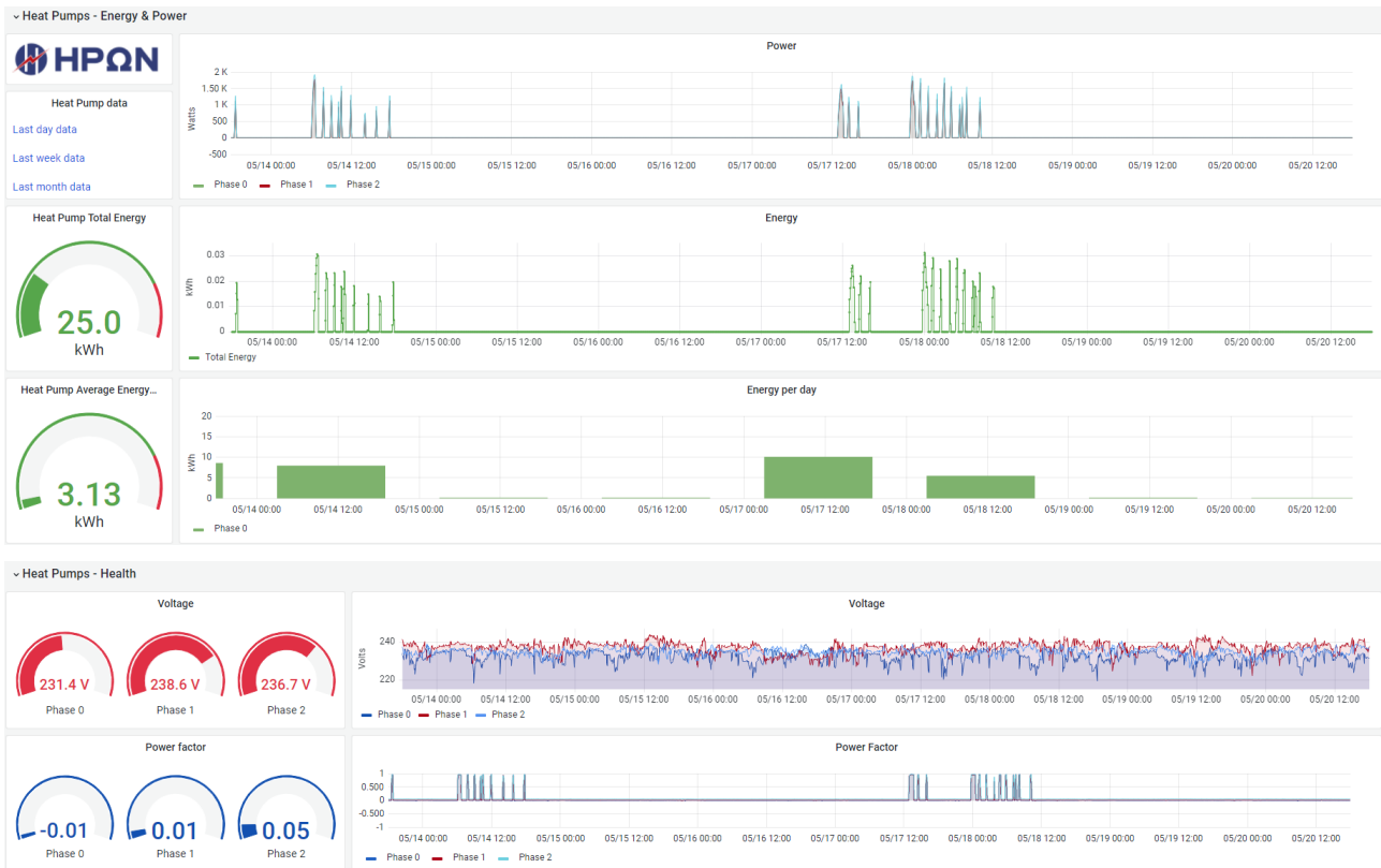
Figure 4: Phase 3 sub-meter measurements (here an example for a Heat Pump).
