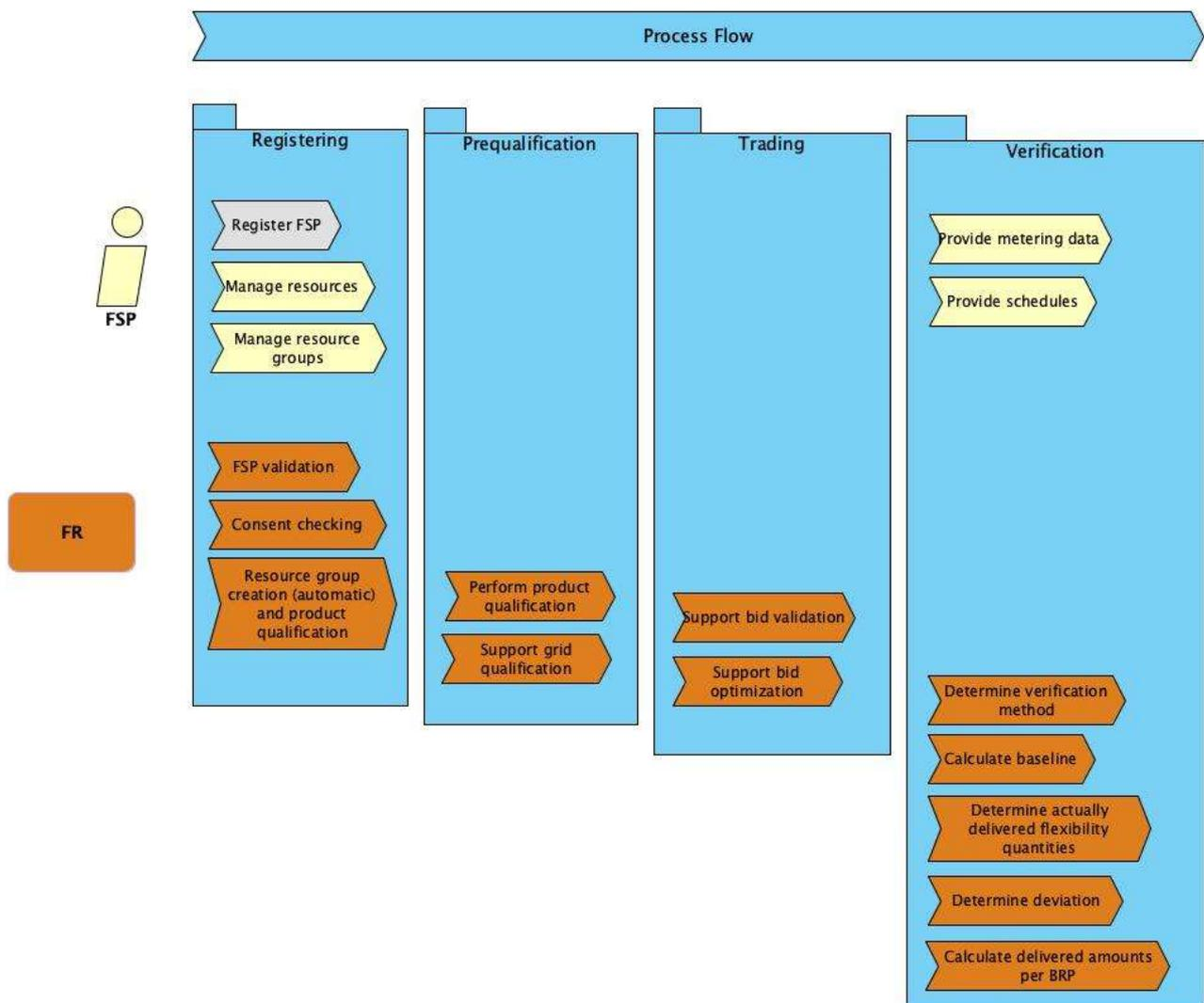
Figure 4-2: Process flow of the Flexibility Register [D7.2]
