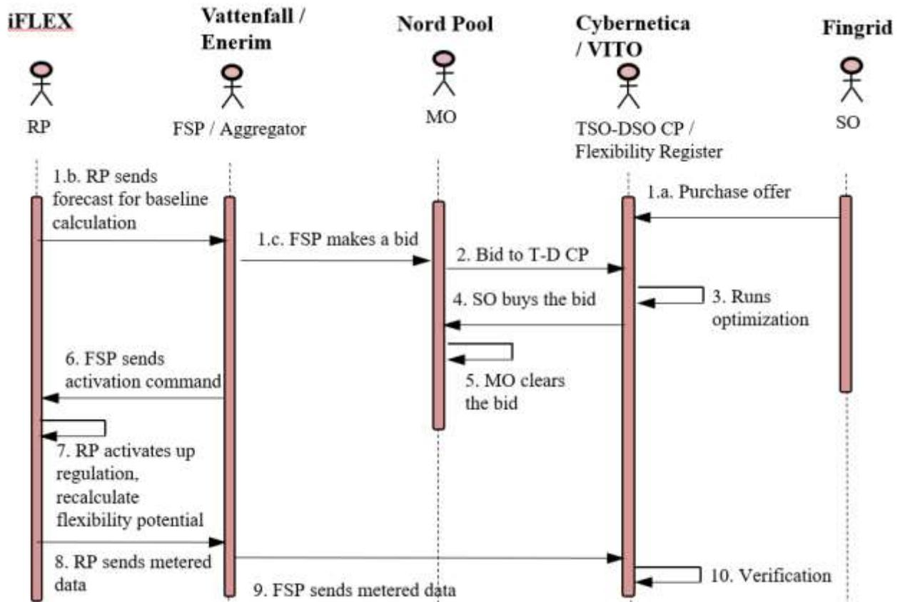
Figure 5-2: Process flow of the iFLEX-OneNet demonstration
