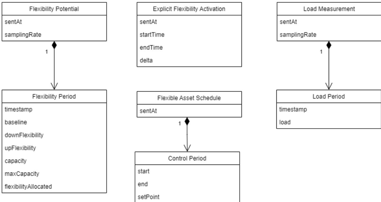
Figure 4-1: Data models for Automated Flexibility Manager interface
