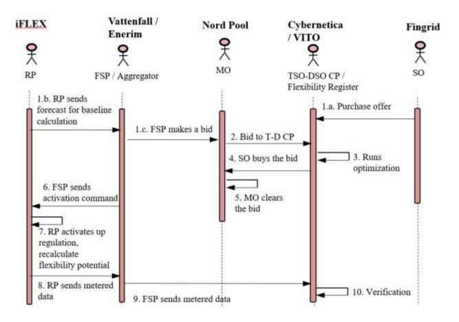
Figure 5-2: Process flow of the iFLEX-OneNet demonstration
